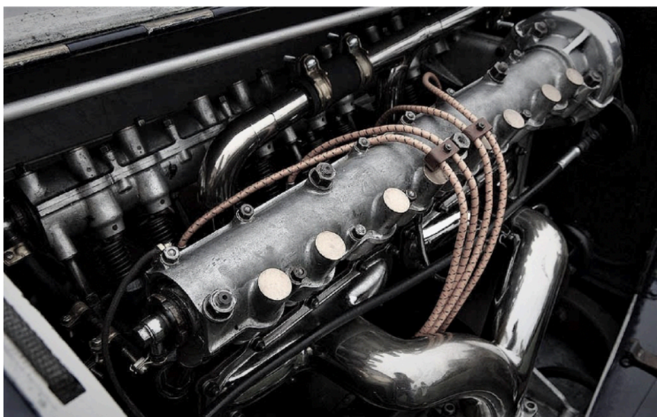
1912 Peugeot L76 engine, the first to use DOHC.
