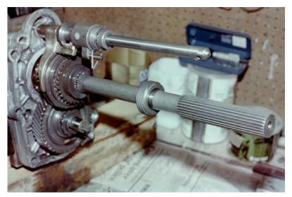
Fitting new speedo drive gearing
