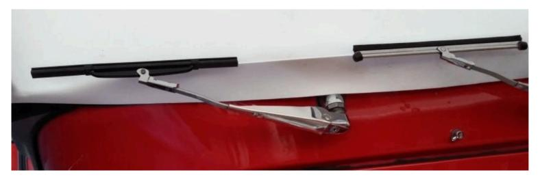
The image above shows both the original wiper alongside the improved version on the left; a sheet of white paper covers the windscreen to enhance the blade image.
