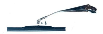
9. Now clip your new assemblies onto the waiting wiper arms on your Mog. There is a photo below of the old and new compared attached. They are resting on a sheet of paper to increase the contrast as they tend to disappear into the darkness on the windscreen. I was able to source the 2.5mm x 10mm stainless screws and locknuts on ebay without having to buy in large quantities.
