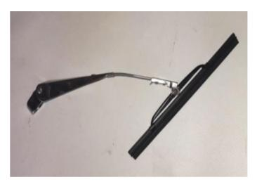
Essentially what I've done is cut down and adapted a Bosch wiper blade intended for a BMW saloon into three Mog sized blades as you can see in the picture below. Any donor blade will do as long as it has the small curved yokes in the pictures.
